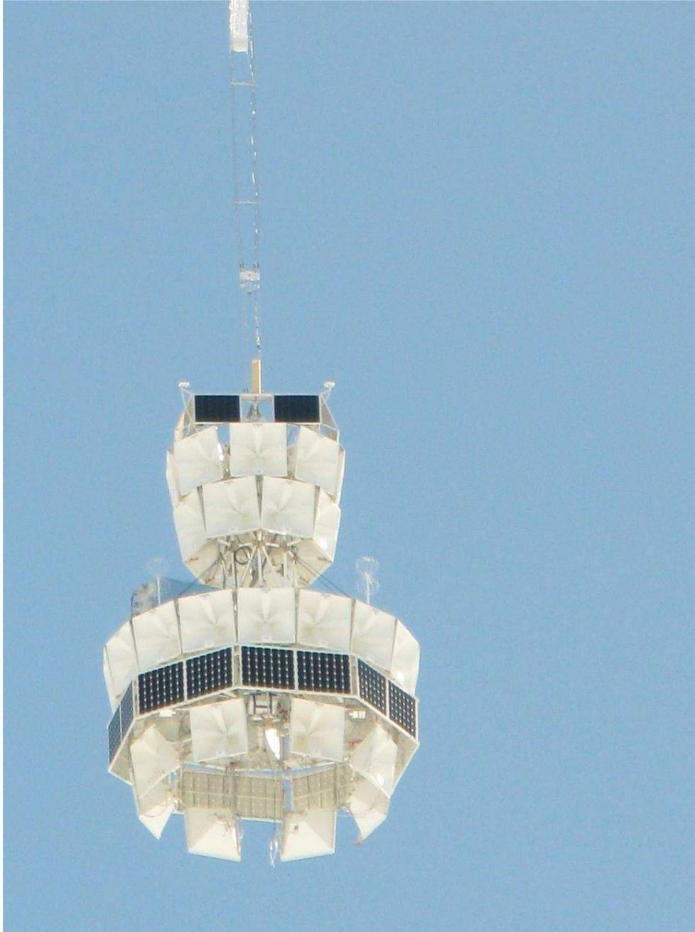
Figure 2.5: A picture of the ANITA-2 payload after launch. The lowest layer of antennas were folded underneath the payload during launch and deployed during ascent. From [54].
